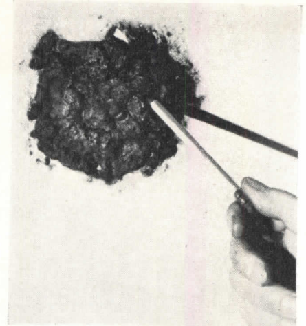
Under blowtorch, special paint puffs out to form protective blanket of insulation
