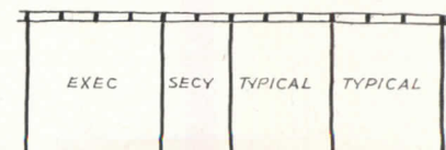
CONTINUOUS FENESTRATION - 4' MODULE SPACING
