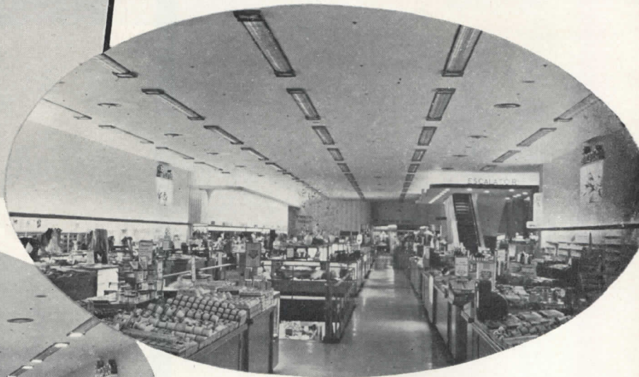
a: Cove lights only: inadequate to do more than provide a background by wall and ceiling brightness.
