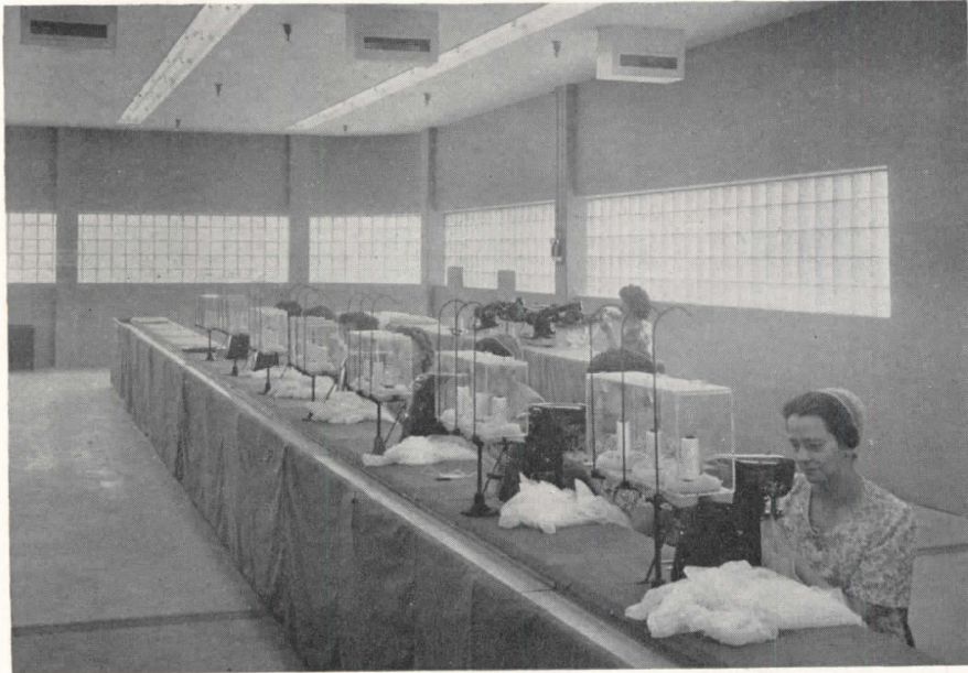
Window openings are sealed with glass block; there are no operating windows. Even with the most precise air conditioning control, looping and seaming operations are carried out under closed covers
