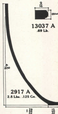
Display case frames are nickel silver and include extrusions from Anaconda dies 2917A and 13037A.
