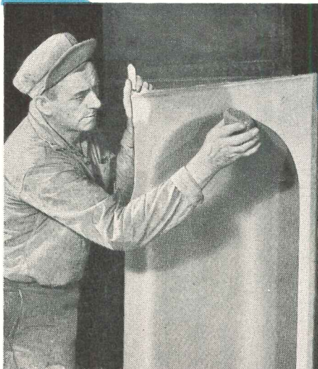
Harold Pickens, with 21 years experience in sandblasting, checks each casting for imperfections. Sandblasting removes sand and foreign materials from the casting and makes it ready for the next step—grinding.
