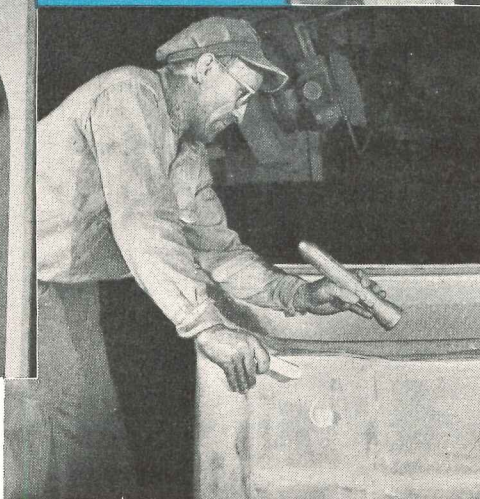
Edward Morva, over ten years a grinding room inspector, carefully examines each casting for any minute roughness or ridges. After his careful inspection proves the casting to be ground perfectly smooth, it is sent on to be enameled.
