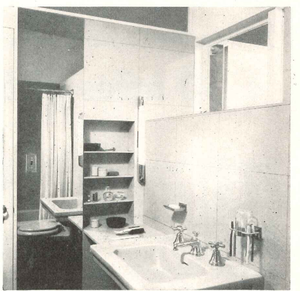
COLORFUL CARRARA STRUCTURAL GLASS is perfect for walls and wainscots of bathrooms, as pictured here. Carrara is mechanically ground and polished. It assures joints that are true and even—without lippage. And it is entirely free of warpage. Available in 10 pleasing colors. Architect: Marcel Breuer, New York City.
