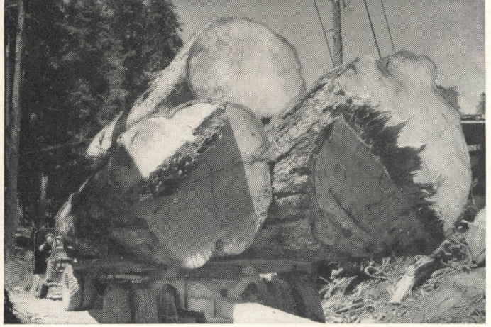
Loads weighing up to 125 tons are carried in one trip on mammoth Weyerhaeuser truck units. Some have two trailers in tandem, making a carrier 100 feet long.
