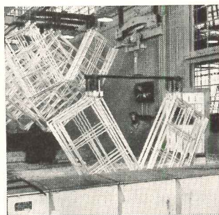
GALVANIZING. Assemblies dip deep into molten zinc, and come up with a heavy, smooth, uniform coating. Temperature and timing are automatically controlled with laboratory accuracy.
