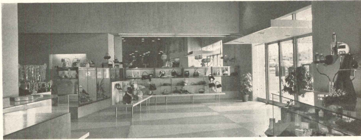
Lower walls are of Travertine marble; upper walls in painted concrete with wide grooves delineating a modular pattern
