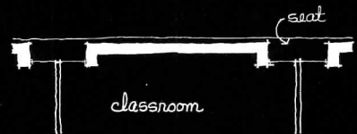
plan section of exterior wall
