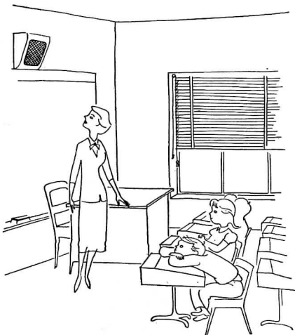
CLASSROOM speakers may have a talk-back feature, working through the monitor speaker on the panel at the control center
