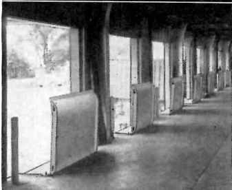
MORE USABLE DOCK SPACE —boards swing up and out of the way . . . occupy minimum space in stored position.
