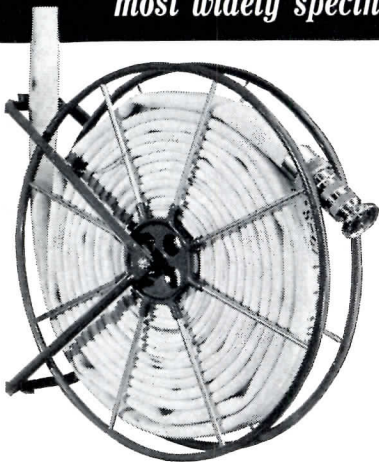
Fig. 145 (UL and FM listed and approved)—Ryerson swinging hose reel with wall brackets or pipe clamps. Holds 50-100-150 feet of cotton rubber-lined hose out of way, yet swings and feeds instantly. To suit type, size and length of hose required.
