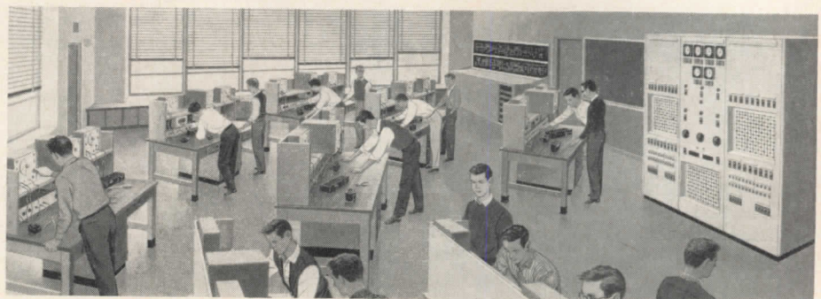
Left: Student benches include equipment needed for carrying out experiments and building model circuits. Below: Typical lab layout ranges task areas around central power unit at right
