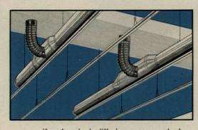
. . . or if preferred, air diffusing vanes may be installed (at factory or in the field) in Main-T and Cross-T members and air supplied with round, rectangular or triangular snap-on ducts.
