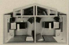
Model of patients room, above, shows concept of accessible toilet at perimeter. Floor-to-ceiling window enhances adjacent sitting area Bedside control of a two-tier drape would seem desirable. Executed concept is below.
