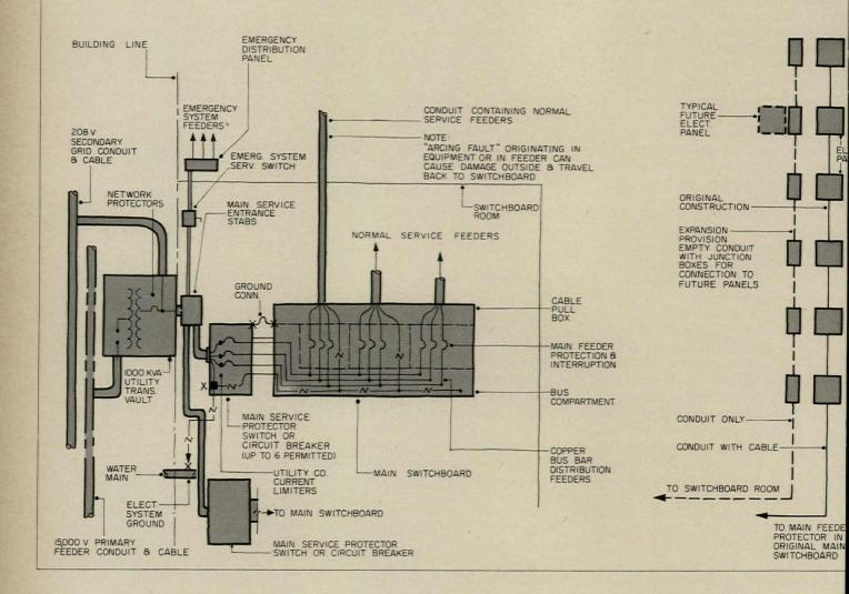
magnitude. While the initial current value of the arc may be small, it will gradually increase as the heat develops, extending the destructive effect back to the main feeder protective device, switchboard and main service switch or breaker.
