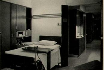
Bedside console has washbasin, locker, cabinet and pull-out electronic controls for radio, TV, drapes, nurse call, etc. Within reach are grab bars to toilet two paces away.
