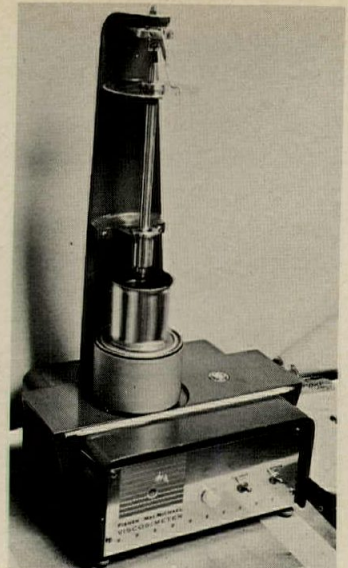
Viscosity of polysulfide sealants is tested to assure that a particular formulation will flow properly from the gun into the joint.
