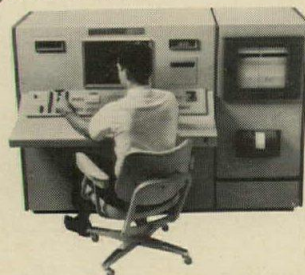
Standardized System 7 Selectographic Supervisory Data Center, with system analyzer and alarm printer module.
