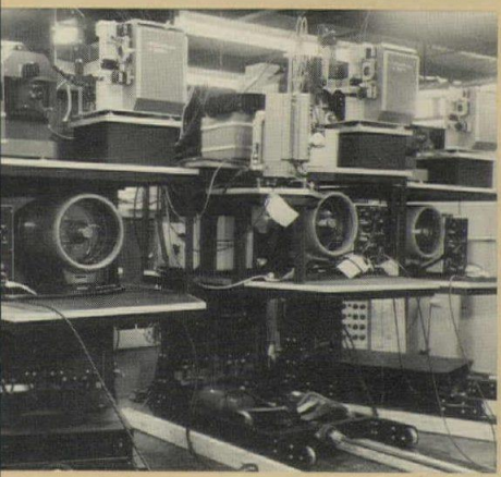
Sophisticated rear screen projection equipment for NASA conference room's multiple screen is mounted in "stories" on three vertical elevator tables. Remote control raises and lowers stories to centerline. The structures on floor tracks can be positioned for one, two or three image projection.
