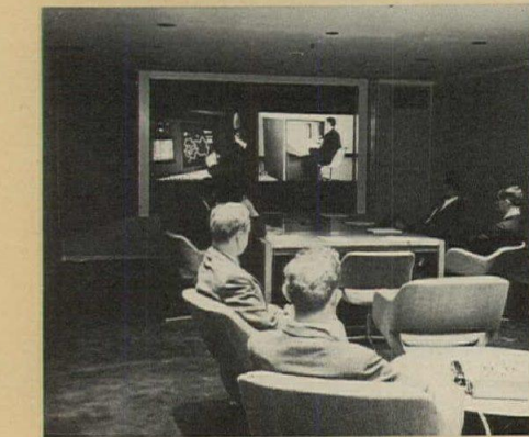
Rear screen equipment for a typical conference room, top photo, includes 16mm movie and slide projector. Mirror inverts movie image for transmission through screen. Participant in a seminar, bottom photo, uses chalkboard, with slides projected on dual-image screen. Rear projection both permits full room lighting and eliminates screen shadows. Equipment can be operated from remote control panel, lower right.
