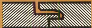
12" x 12" x 1/2" Self leveling tile for metal suspension systems, staple or adhesive application.
