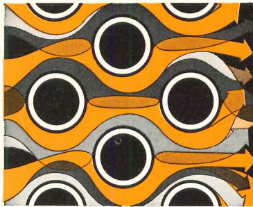
McQuay's staggered tube design eliminates dead spots behind tubes
