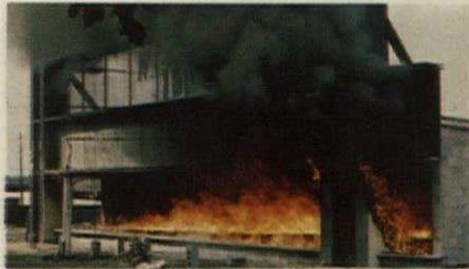
To prove that flame-shielding works, tests were conducted on a full-scale mock-up.
