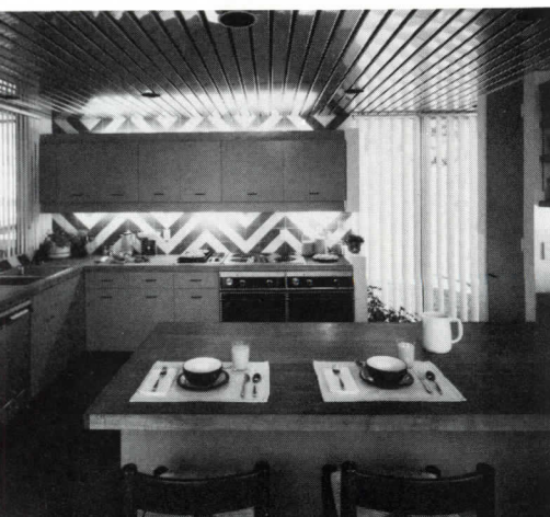
The translucent roof is supported by aluminum box beams, the longest spanning 42 feet. Aluminum is also the finish for the suspended ceiling in the kitchen (photo left). The kitchen's end wall is finished in chevron-patterned tile.
