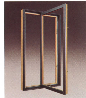
Pella's Clad Casement has a unique hinging system which moves the sash to the center of the frame as the window is cranked outward. This wide open position provides plenty of room to clean outside glass from inside.
