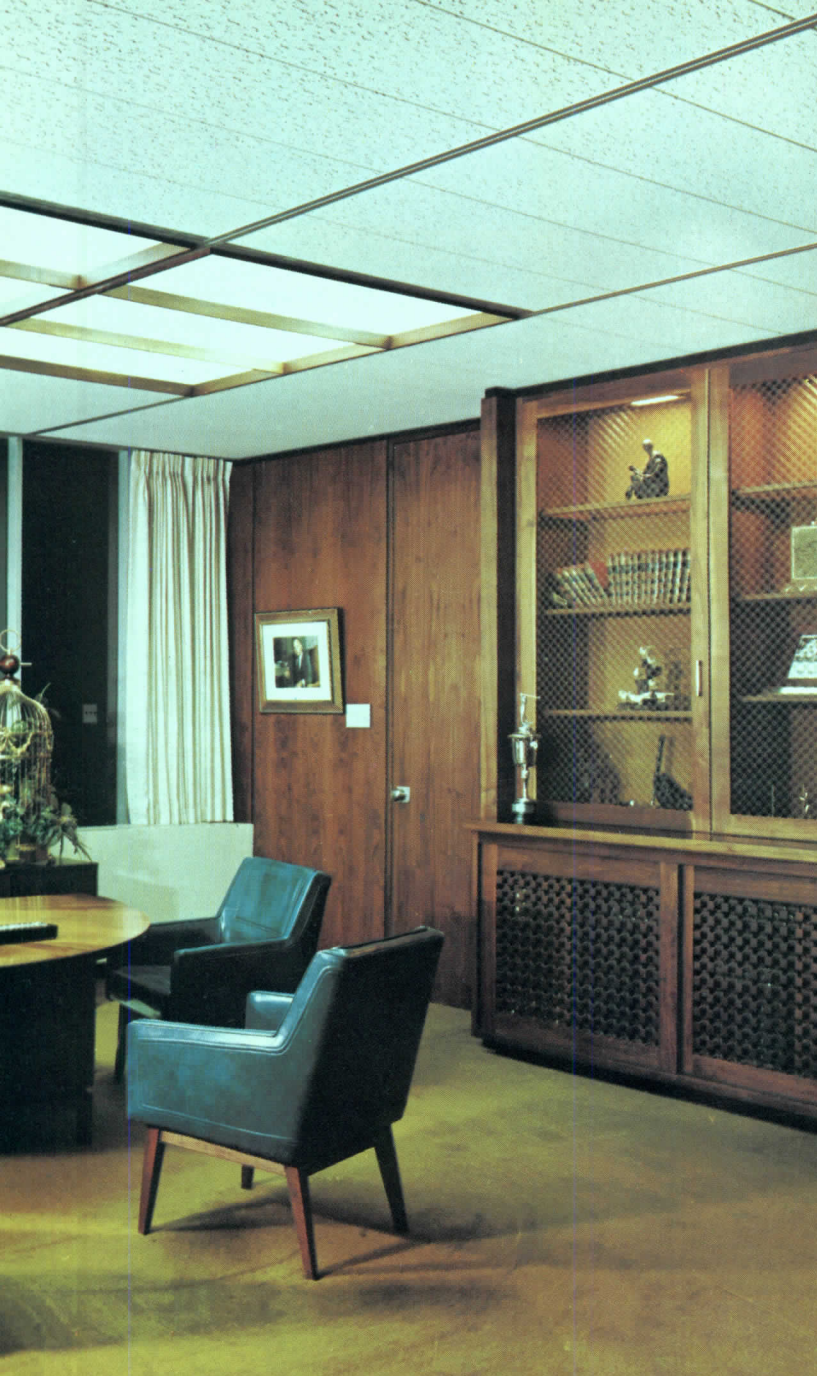
Solitude Tile (5/8" x 12" x 12") is beveled, kerfed and rabbeted . . . designed for installation with a concealed spline suspension system, or with adhesive.
