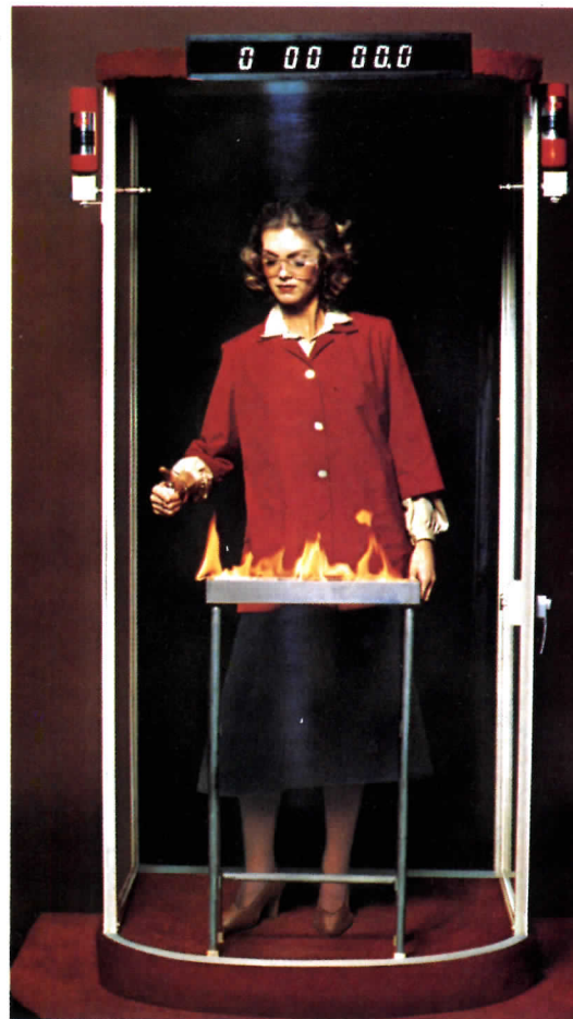
1. Flammable liquid ignited. Halon 1301 cylinders discharged.
