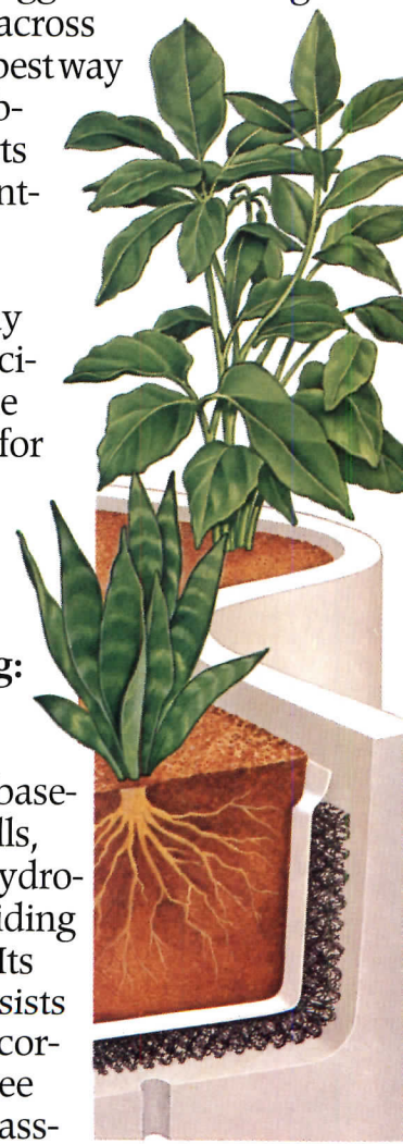
Enkadrain "pulls" roots to the sides of the planter for fuller development, as it encourages lateral drainage. (See Sweet's 2.7d/Ame)
