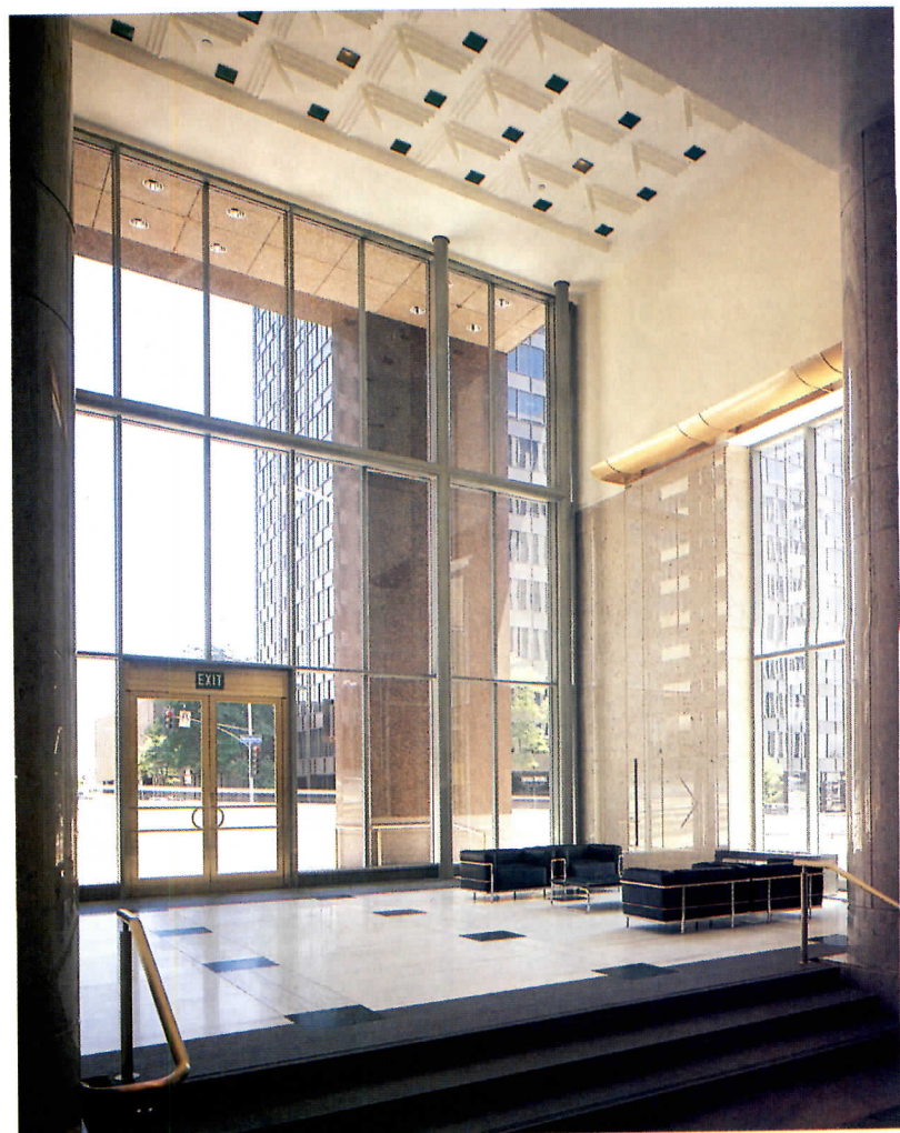
The Wilshire Boulevard lobby rises 33 feet to a coffered ceiling made of glass-fiber reinforced plaster. Square green-glass lenses in the ceiling conceal incandescent fixtures.
