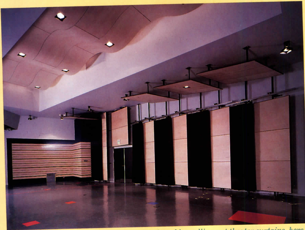
The reverberation time of the room can be altered by pulling out theater curtains, here shown in the half-open position.
