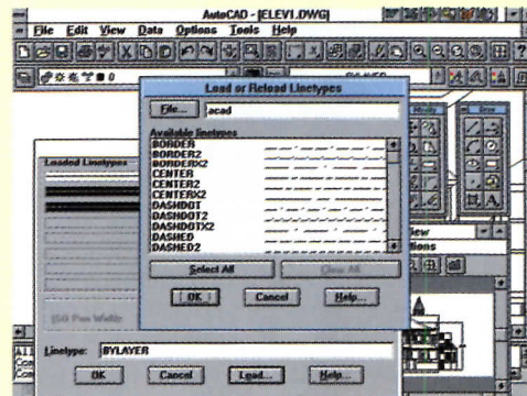
These are among the linetypes that come with Release 13. You can also create your own—similar to MicroStation.
