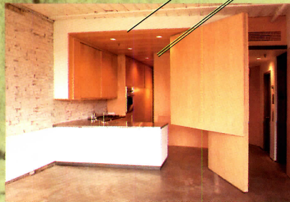
By tucking a kitchen, sleeping loft, and bathroom behind a pivoting partition (sketch and
