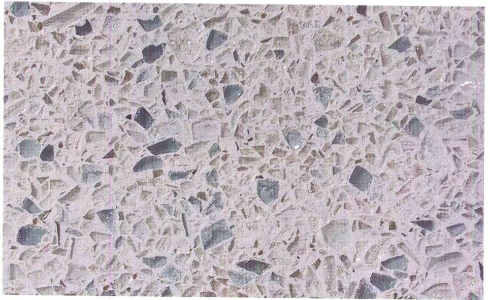
Milky white epoxy is mixed with recycled glass to form a terrazzolike floor for IBM's E-business Center for Innovation in Chicago. The finish has more visual depth than conventional terrazzo.
