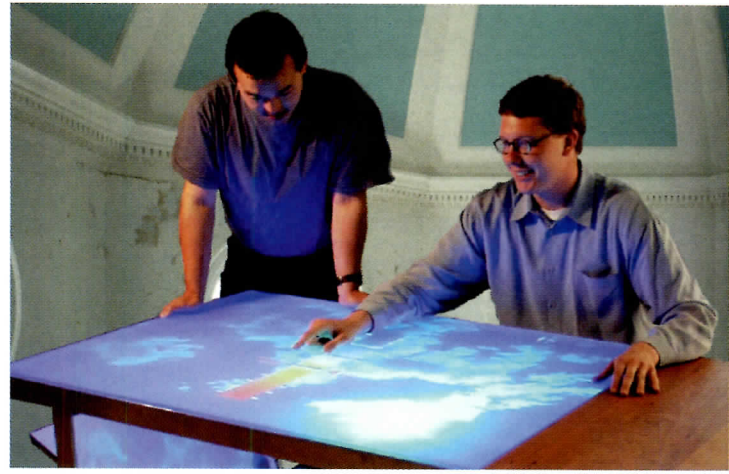
Students Byron Stigge and Tyron Yang made a horizontal-display prototype to help home occupants monitor and plan energy conservation.
