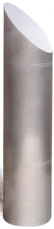
Above: Metropolitan Bollard: Round Stainless Steel or Bronze Satin Finish Size: 48" high x ?? diameter Custom sizes available Pipe Size: 8" Schedule 80 pipe (to be filled with concrete)
