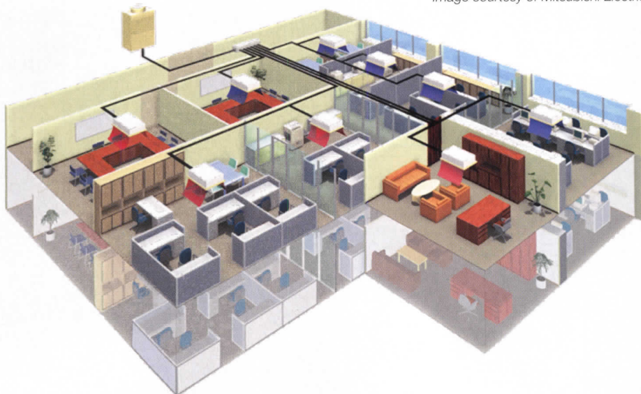
VRF systems include a central variable capacity outdoor unit connected to multiple variable capacity indoor units.
