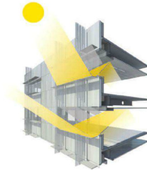
EDITH GREEN/WENDELL WYATT FEDERAL BUILDING: LIGHT REFLECTOR AND SUNSHADE DIAGRAM
