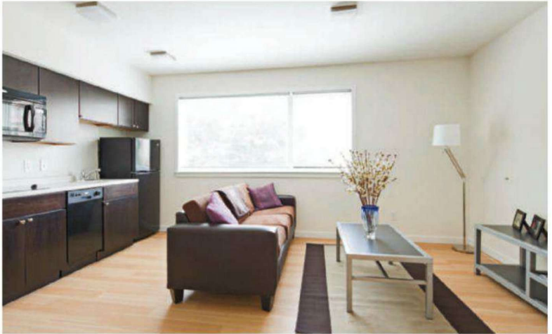
FINISHES FIRST The prefab units shipped with interiors nearly completed. Interface selected from a list of the manufacturer's preferred finishes—custom specifying only the flooring and light fixtures.
